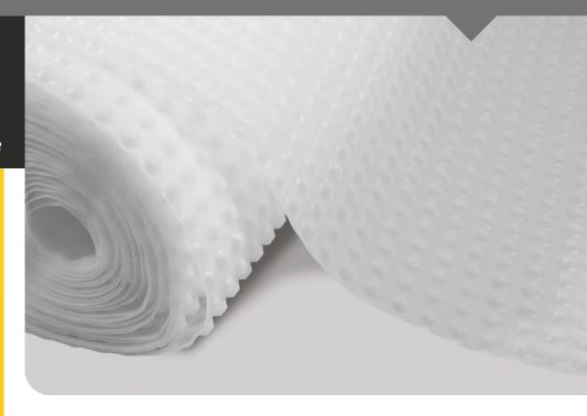
**CM8 HD** is an 8mm studded high density membrane suitable for type C waterproofing and delivering a grade 3 environment to BS8102:2009 and NHBC chapter 5.4. We recommend using the HD version on our Danopren insulated spacer and also in commercial areas where a more impact resistant membrane may be needed. CM8 HD is also an excellent Radon barrier and has passed all the relevant tests for resistance to this Gas.
