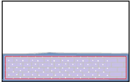
Lift back membrane edges and insert sealing Rope between membrane and wall/primer
