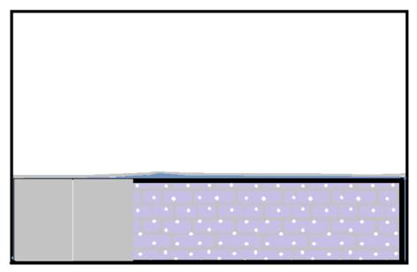
Fit plasterboards ensuring dabs hit membrane fixings
