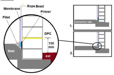
If concrete floor cut a small fillet from edge of floor slab(use diamond bladed grinder) and fit membrane to bottom of fillet
