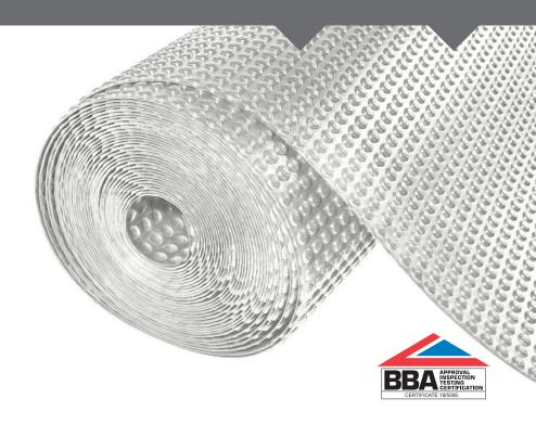
**CM3 Cavity Drain Membrane** is a 3 mm studded membrane, suitable for Type C waterproofing or damp-proofing, and delivering a grade 3 environment to BS8102:2009 and NHBC Chapter 5.4.
