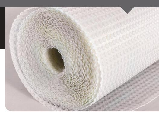
**CM3 Cavity Drain Mesh Membrane** is a 3 mm studded membrane incorporating a tough HDPE mesh lathing welded to the front face, allowing the direct application of various plaster finishes, adhesive 'dabs' and plasterboards and delivering a grade 3 environment to BS8102:2009 and NHBC Chapter 5.4.
