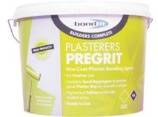
An alternative for these surfaces is to use Bond It PREGRIT or to mix 1 part PVA ADMIX:1 part water and use to slurry a blend of 1 part Portland cement:2 parts clean sharp sand and apply with a notched trowel. Allow to dry for a minimum of 24 hours and then apply a top coat of plaster or cement.
